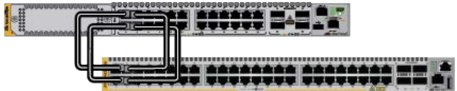
Stack of Two Switches
