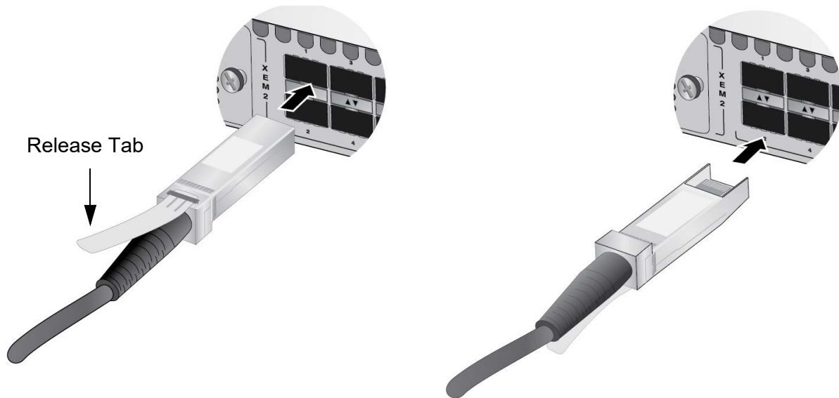
Figure 136. Installing SP10TW Direct Attach Cables
