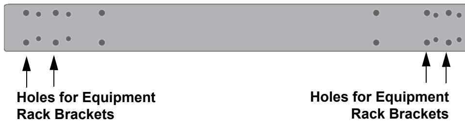
Figure 85. Holes for the Equipment Rack Brackets on the x950-52XSQ and x950-52XTQm Switches
