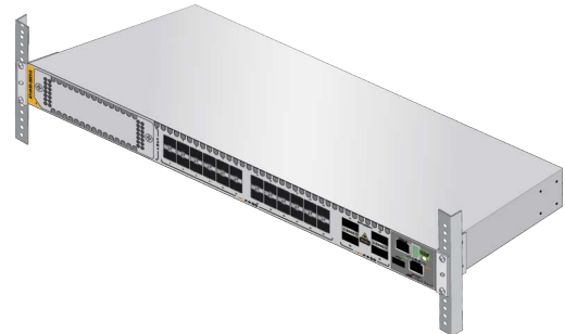
19-inch Equipment Rack with Standard Brackets
